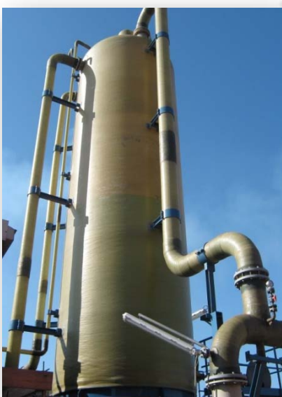
VERTICAL TANK De 3000 h.13000 in PRFV
